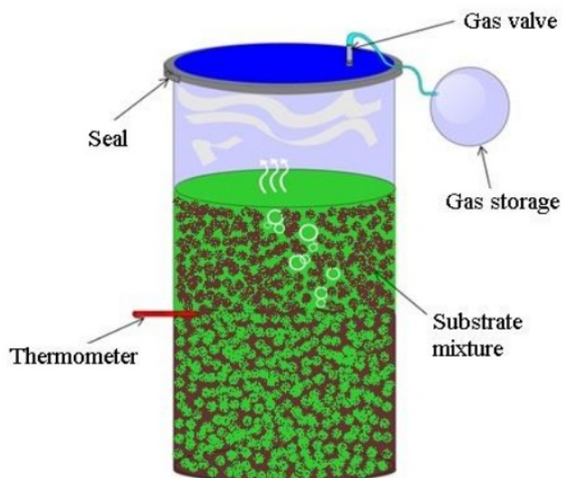
Fig. 1 A 220-L drum digester prepared for the experiment
