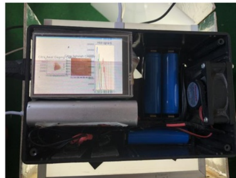
Fig. 5. Display Image Processing on Raspberry Pi screen
