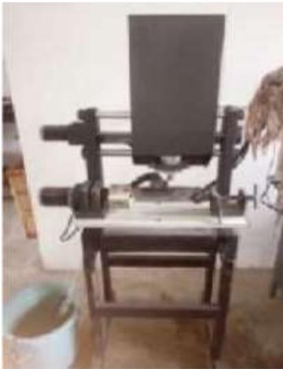
**Gambar 3.** Mesin cnc micro-milling
