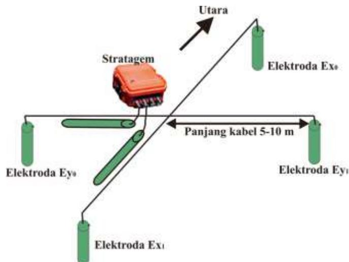
**Figure 2.** The installation of the stratagem AMT tool as the center by burping the electric electrodes in the north-south direction on the x-axis, and the magnetic coil on the y-axis oriented west-east with a stretch cable of about 5-10 m.
