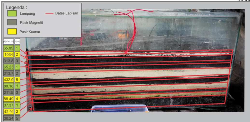
Figure 1 The original resistivity value of each layer in the horizontal layer model
