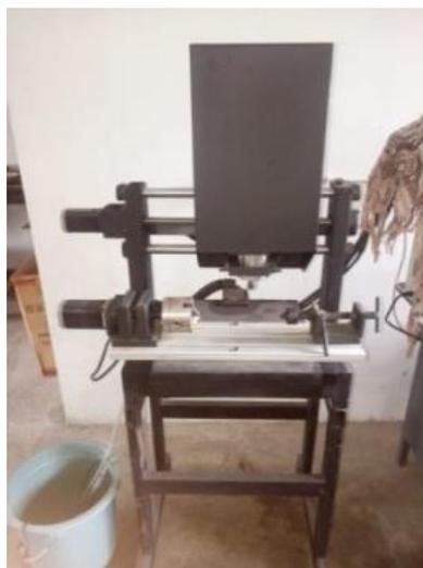
**Gambar 3. Mesin cnc *micro-milling***
