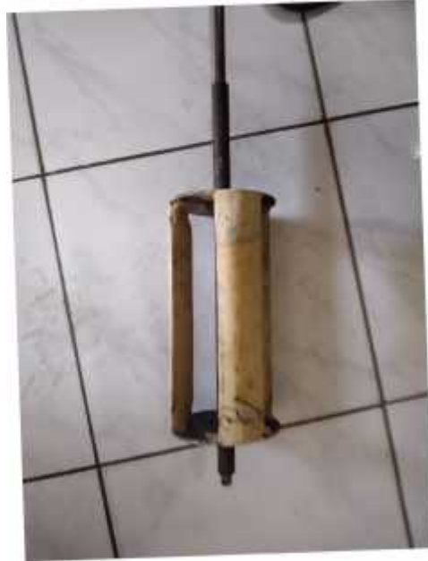
Figure 8. Model of hydrokinetic turbine with three blades
