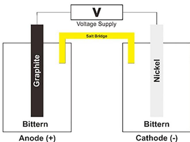
Figure 1. The electrochemical set-up used in this study.
