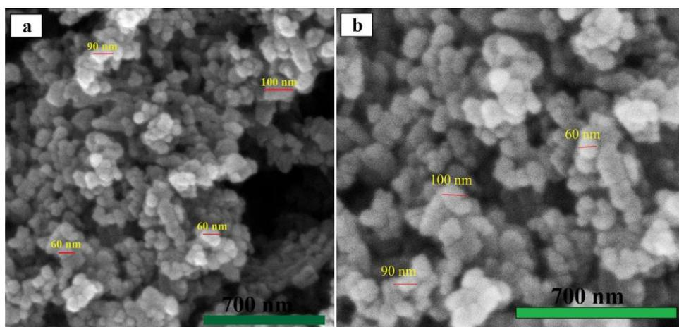
Figure 6. SEM micrographs of synthesized MgO samples: (a) seawater; (b) bittern.
