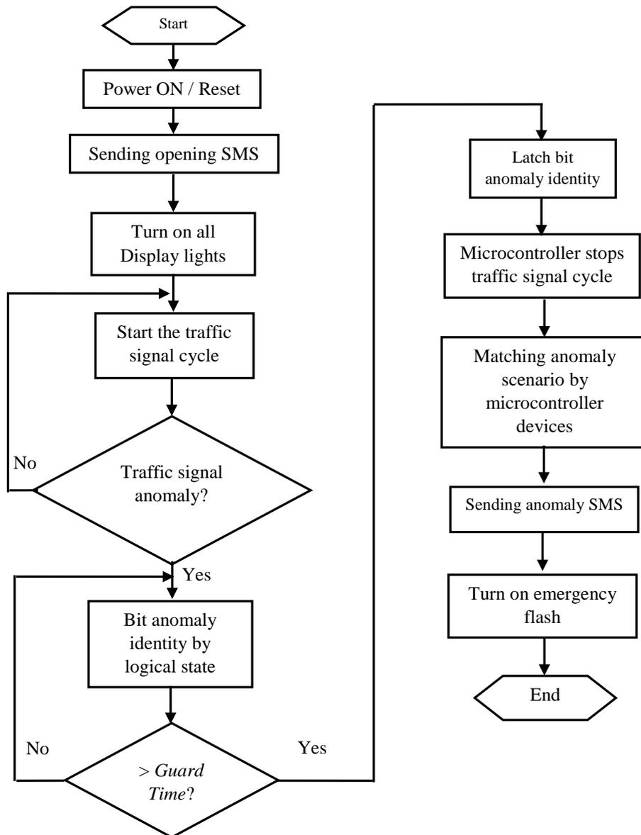
Fig. 4 Flow chart of signal monitoring system
