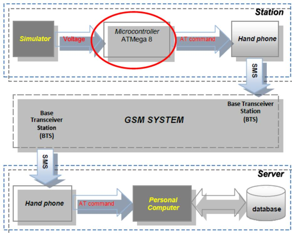
Fig. 5 Self-diagnosis system of traffic light [7]
