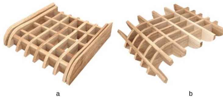
Figure. 3. Illustration of bottom (a) and upper (b) press mold part used to shape the laminated bamboo material using the Two-way Press system
