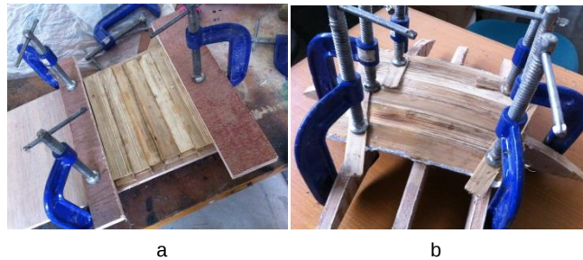
Figure. 5. Experimental process of press mold for seat component of bamboo chair
