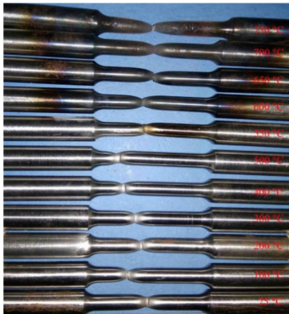
Fig. 16. Failure modes of CDS AISI 1018 specimens after high-temperature tension testing under steady-state conditions.
