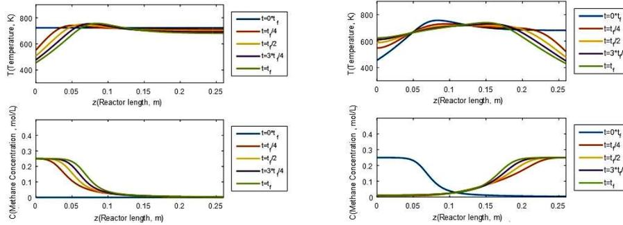
**Figure 1.** Temperature and concentration behavior of feed gas for various time values  $t$  with  $A = 0.25$ ,  $\varepsilon = 0.05$  and  $\omega = 0$ . Left figure, for flow from left to right and right figure after reversed.
