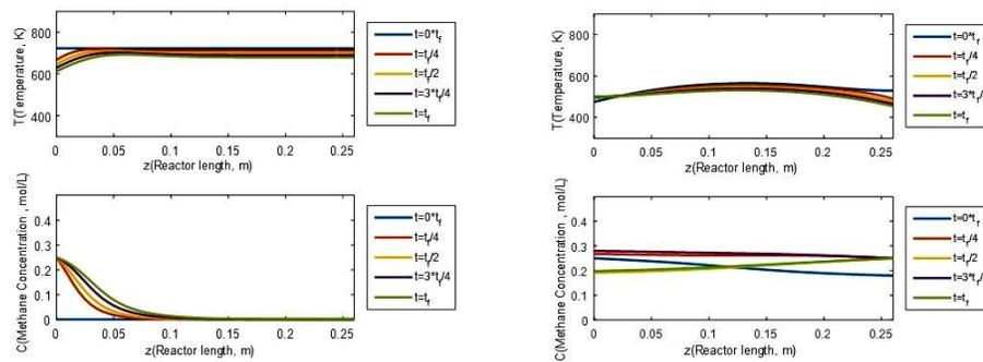
**Figure 6.** Temperature and concentration behavior of feed gas for various time values  $t$  with  $A = 0.25$ ,  $\varepsilon = 0.05$ ,  $u = 0.1$  after six times reversed. Left figure, for  $\omega = 5\pi$  and right figure  $\omega = \frac{\pi}{5}$ .
