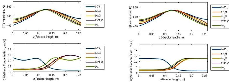
**Figure 3.** Temperature and concentration behavior of feed gas for various time values  $t$  with  $A = 0.25$ ,  $\varepsilon = 0.05$  after six times reversed. Left figure, for  $\omega = 5\pi$  and right figure  $\omega = \frac{\pi}{5}$ .
