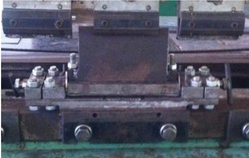
Figure 1. Experimental Methods for Embossing on Fin Wheel Using Bending Press Brake V
