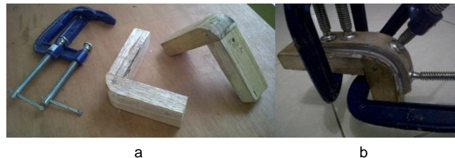
Figure. 6. (a) wooden molds for bending the seat frame structure (b) bending process frame structure of bamboo chair
