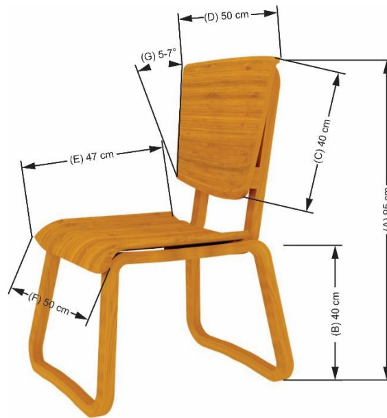
Figure 7. Design and measurements of bamboo laminated chair which conforms to anthropometric standards
