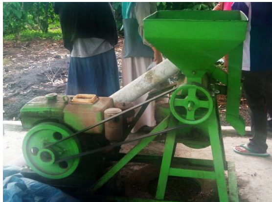
Figure 5. Postharvest treatment equipment: pulping machine.
