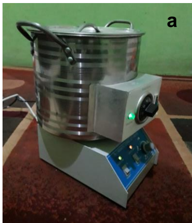
Figure 6. Heating process, portable water bath paired on magnetic stirrer.
