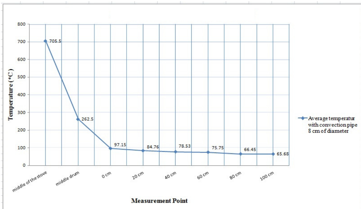
Figure 6. The average temperature at each drum point using convection pipes of 8 cm.
