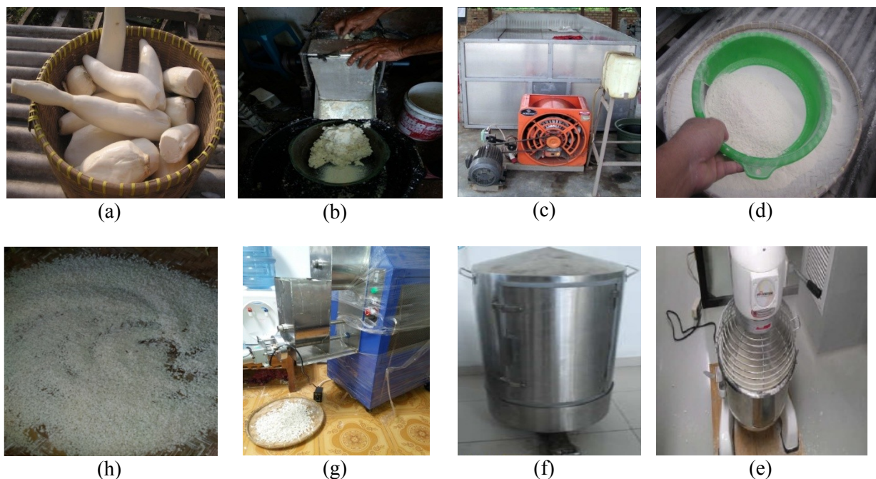
Figure 2. The process of making siger rice from waxy cassava. (a) cassava tuber, (b) grinding, (c) drying, (d) sieving, (e) mixing, (f) steaming, (g) extruding, and (h) siger rice
