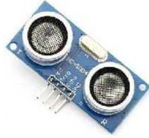
Gambar 3. Sensor ultrasonik HC-SR04.
