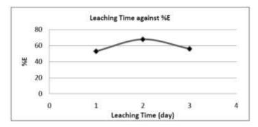
Figure 3. Mean effect plot for leaching time against the percentage of nickel extraction
