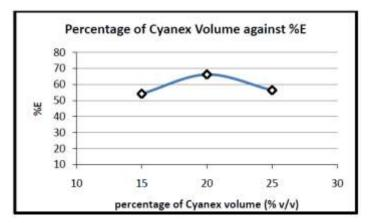
Figure 4. Mean effect plot for the percentage of the cyanex volume against the percentage of nickel extraction
