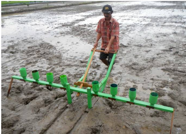
Gambar 1: Alat tanam benih padi langsung tipe manual slide hopper
