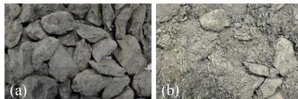
Fig. 1. Slaking of crushed mudstone (a) initial condition and (b) after slaking (an example of the accelerated slaking tests).
