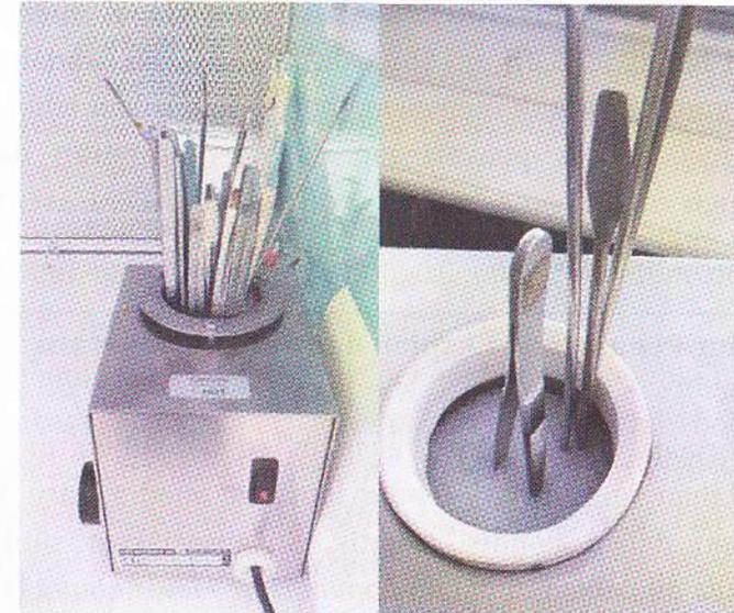
**Gambar 8.3** Contoh *glass-bead sterilizer*, alat pensteril alat-alat diseksi
