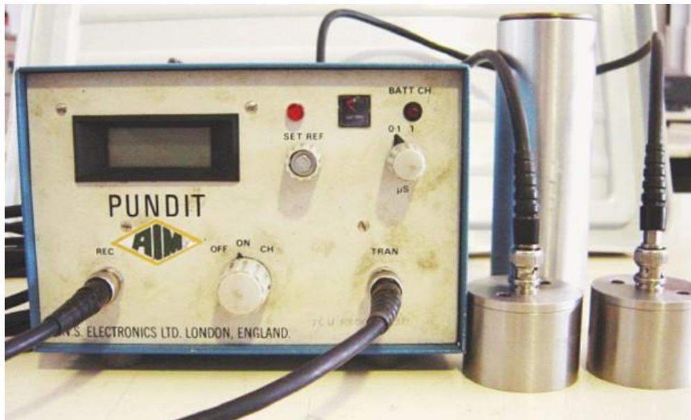
Gambar 3.1 Uji Non-destructive dengan Portable Ultrasonic Non-destructive Digital Indicating Tester.
