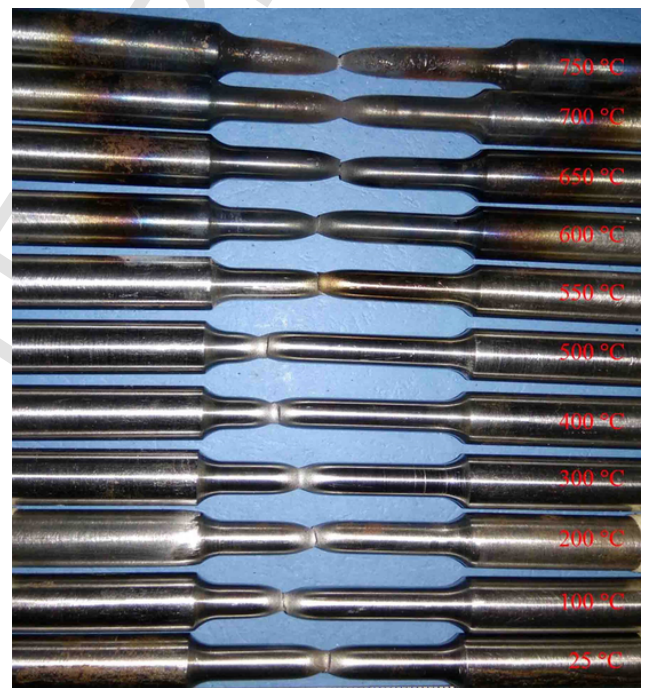
Fig. 16. Failure modes of CDS AISI 1018 specimens after high-temperature tension testing under steady-state conditions.
