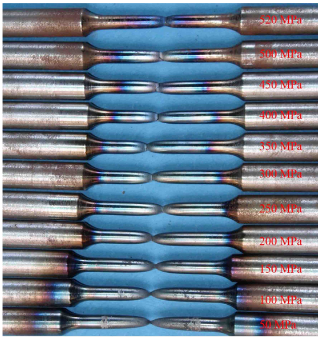
Fig. 17. Failure modes of CDS AISI 1018 specimens at different stress levels after transient temperature deformation tests.
