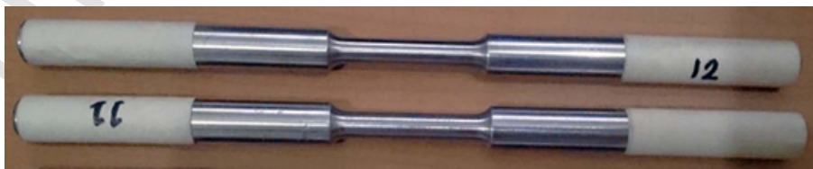
Fig. 2. Photographs of the tensile specimens.
