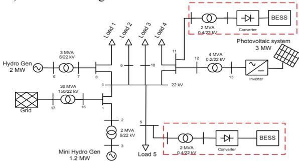
Figure .7. The BESS installations at local substations
