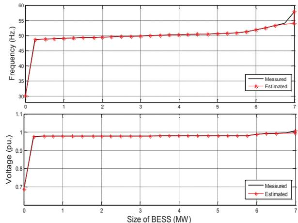
Figure. 9. A comparison between measured BESS size and predicted BESS size based on frequency and voltage control of the micro-grid
