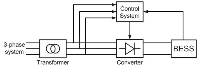
Figure 2. A structure of BESS [7]
