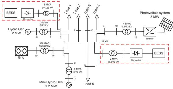
Figure. 5. The BESS installations at a main and local substation
