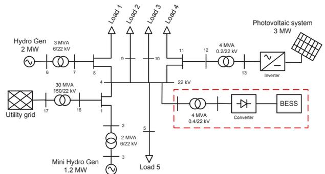
Figure 4. The BESS installation at a main substation
