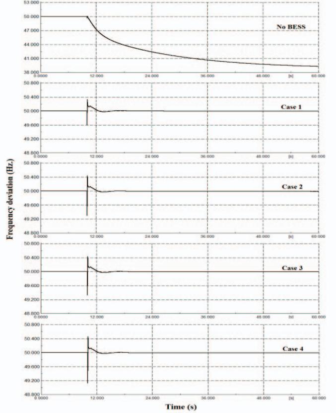
Figure 11. Frequency deviations for different cases after islanding
