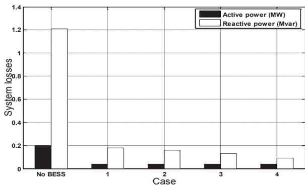
Figure. 13. A comparison of system losses for different BESS locations
