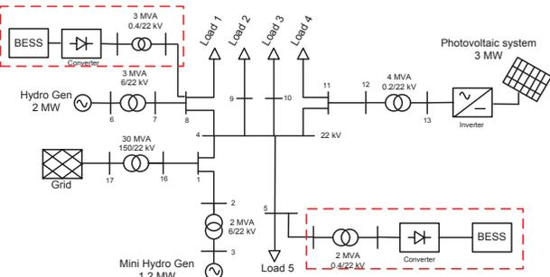
Figure. 6. The BESS installations at local substations
