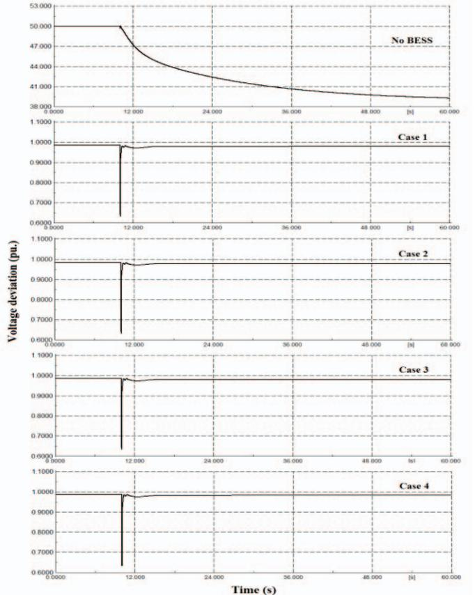
Figure 12. Voltage deviations for different cases after islanding
