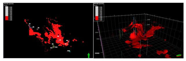
FIGURE 7. Coal seam A distribution from relative density cut-off 1.4 gr/cc
