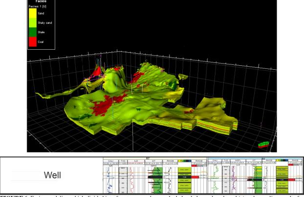
FIGURE 6. Facies modeling which divided into four types, such as coal, shale, shaly sand, and sand (a) and upscaling results for coal seam A in two wells (b)
