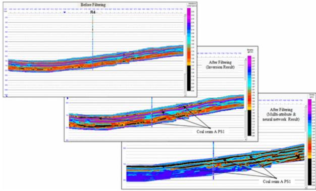
**FIGURE 5**. Seismic inversion results featuring the coal seam A PS-1 before filtering (above), after filtering (middle), and after a multi-attribute and neural network (below) with cut-off density value of coal (black layer) <1.4 gr/cc.
