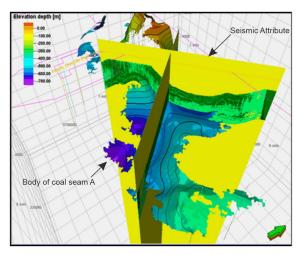
FIGURE 8. Cross-check body of coal seam a with a seismic attribute and to validated 3d modeling coal seam A
