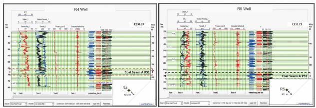
**FIGURE 4.** The results of the well seismic tie in R4 (left) and R5 (right) well that produced correlation about 0.87 and 0.73 with a red dashed line is the coal seam target.
