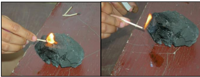
Fig. 11. Combustion test on organic clay and organic carbonate
