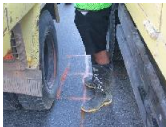
Figure 13 Position of rear wheel of truck on loading of combination 2
