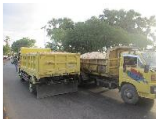
Figure 11. Two trucks at loading position on box-girder bridge that tested.
