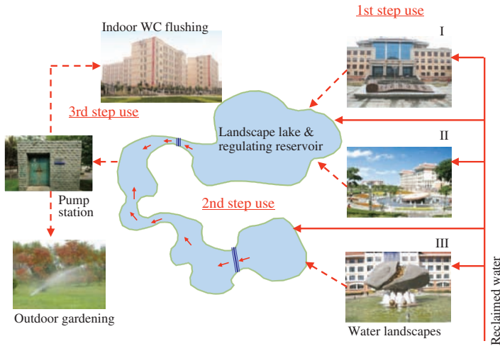
Figure 5.11. Landscaping lakes in the water cycle for stepwise water use, water storage and water quality improvement
