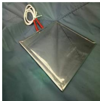
Figure 3. A plate heater
