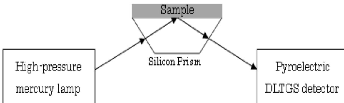
Figure 1. The schematic diagram of spectral measurement using ATR-THz spectroscopy.
