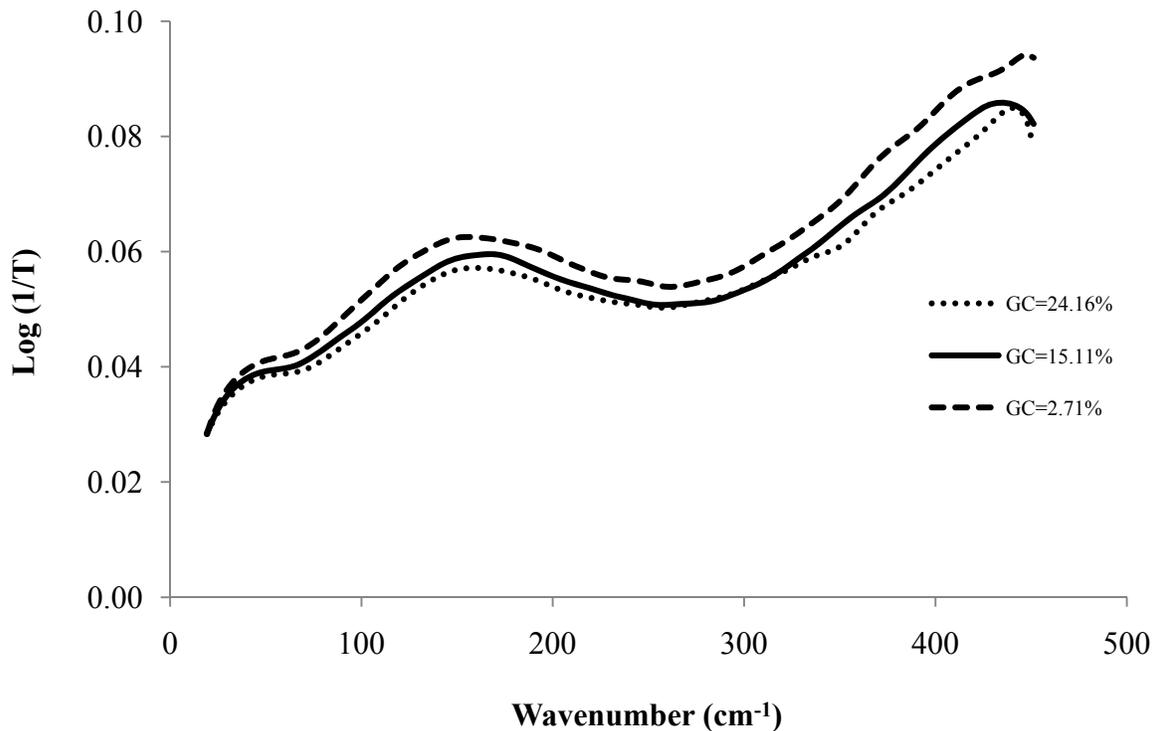
Figure 2. Typical ATR spectra of glucose solution with different concentration in THz region.
