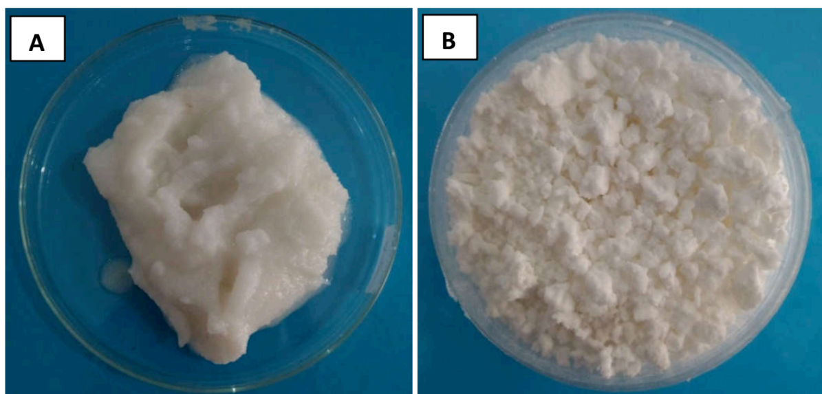
Figure 2. Mg(OH) 2 product (A) wet, (B) dry. “all dilution factors give an identical product morphology”
