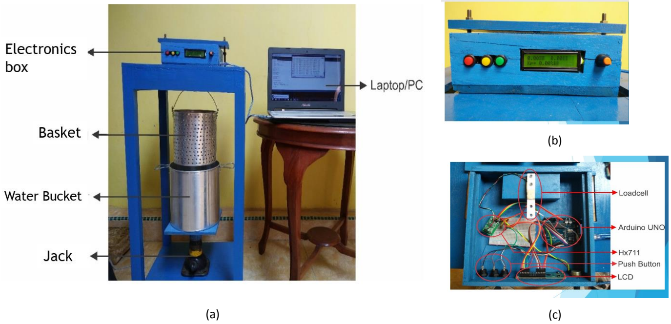
Figure 3. a) Complete instrument for measuring starch content. b) LCD screen panel. c) Top view of the electronics box.
