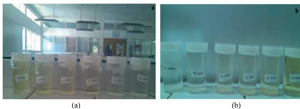
Figure 9. Dye photodegradation results under visible light irradiation (a) and ultraviolet (b) for 0–50 min.
