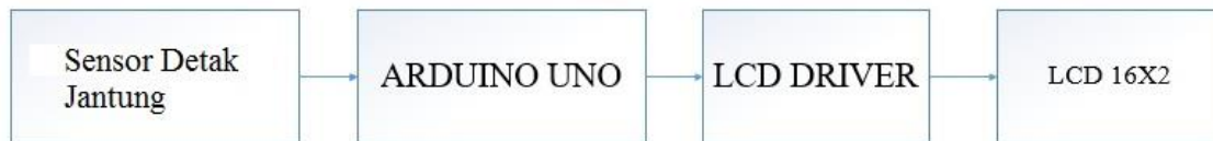
Gambar 5. Blok diagram system alat ukur
