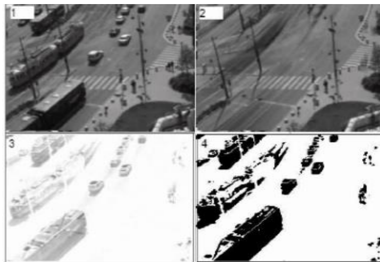
Gambar 1. Background subtraction -1 gambar awal, 2- background model , -3 hasil background subtraction , -4 hasil background subtraction setelah threshold
