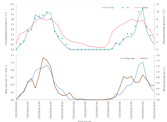
Fig. 4 Time Course of the net photosynthesis, transpiration and vapor pressure deficit (upper); wind speed and ventilation flow rate (below) under SV12 without PFC treatments (22-23 July,2018).
