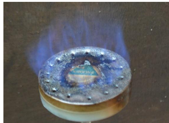
Fig. 4 Burning test for biogas produced from efb through dry anaerobic fermentation.
