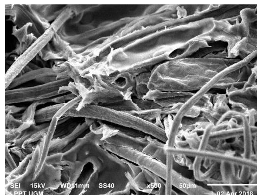
Fig. 6. SEM of unbleached pulp of bamboo-PLA composite (500x magnification)
