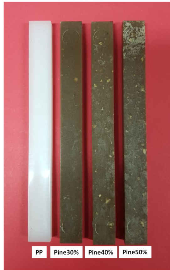
Fig. 6. Images of pure polypropylene and its biocomposite at different loadings of pineapple pulp fiber
