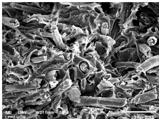
Fig. 7. SEM of bleached-acetylated pulp of bamboo-PLA composite (500x magnification)
