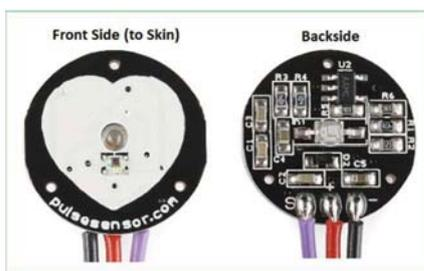
Fig.2 Pulse Sensor
